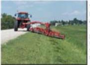
The RCH TM arm technology allows the mower to be moved from left of the tractor to the right with only the push or pull of your hydraulic lever. Imagine the benefits!! You can move around sign posts, cutting right up to them and moving around them. Cut very steep grades on your right or left while your tractor remains level. This NEW design truly is something the industry wanted.
