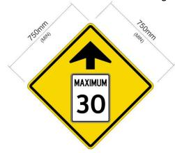
Warning signs must be a minimum of 750 mm along each side and conform to MUTCD requirements.
