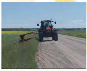
The RCH m arm technology allows the mower to be moved from left of the tractor to the right with only the push or pull of your hydraulic lever. Imagine the benefits!! You can move around sign posts, cutting right up to them and moving around them. Cut very steep grades on your right or left while your tractor remains level. This NEW design truly is something the industry wanted.
