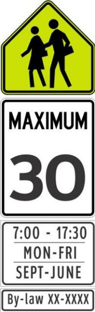
A sign identifying when the speed limit is in effect must: be at minimum 600 mm x 400 mm, be reflectorized and look similar to the sign pictured.
