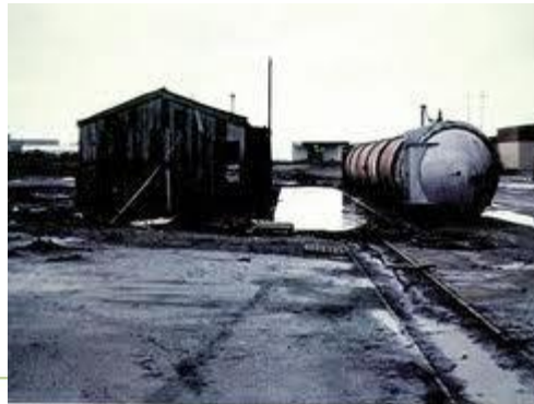
A container used to treat wood with chemicals by saturation.
